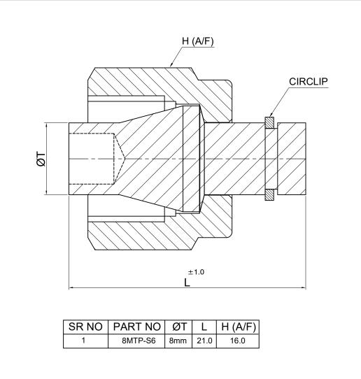
PART NAME: TUBE PLUG CUSTOMER NAME:-PROJECT NAME: - -DWG NO : GA-TP-S6 MATERIAL : SS316 PO NO:-SIGN DATE 12.10.2022 DRAWN BY SHEET NO: 01 OF 01 ENQ NO: EN2223/00815 CHECKED BY 12.10.2022 SB APPROVED BY SM 12.10.2022 SO NO: -DESCRIPTION SIGN DATE \* All dimensions are in mm. Dimensions for reference only and are subject to change without notice
