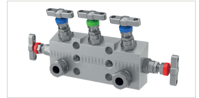
5-valve direct mount manifold having the Parker superior advantage input connections provided through inverted tube fitting connections. Vent can also be specified as threaded or PTFree connect™.
