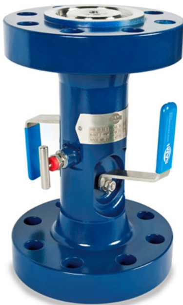
DBB - BALL/NEEDLE/BALL API 10K Inlet: 2 1/16" Outlet: 2 1/16" Material: DUPLEX F51 Painted
